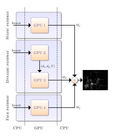
Figure 5.11: Block diagram of multi-GPU pipeline model
