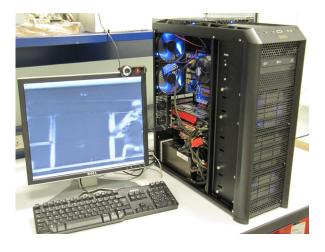
Figure 5.13: Platform for multi-GPU implementation of visual saliency model.
