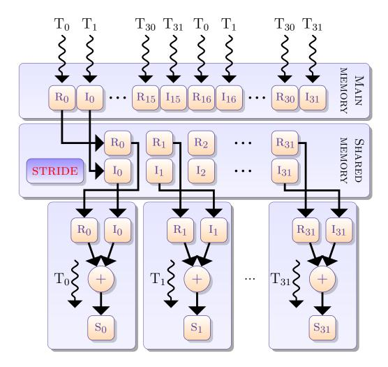
Figure 5.6: Block diagram of data-parallel interaction kernel
