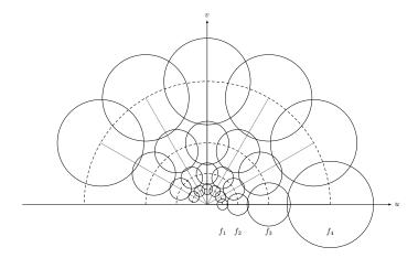
Figure 5.4: Gabor filter bank configuration in the plane (u,v) with six orientations (0°, 30°, 60°, 90°,  $120^{\circ}$ ,  $150^{\circ}$ ) and four frequency bands ( $f_1 = 0.03125$ ,  $f_2 = 0.0625$ ,  $f_3 = 0.125$ ,  $f_4 = 0.25$ ).
